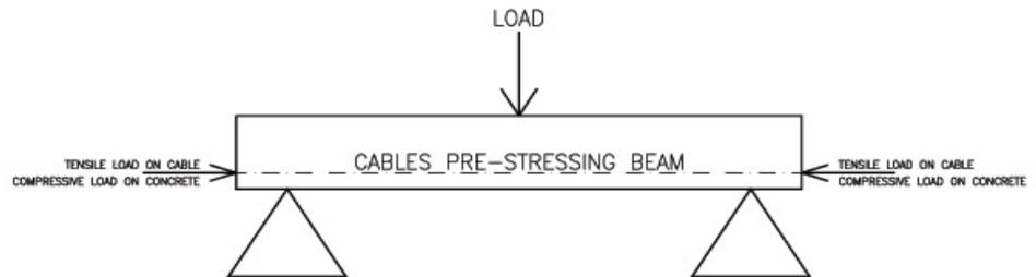
And, one final thought, similar loading can be done after the beam is poured if tubes are left in the concrete for the cables to be stretched in. That is called post-tensioning, rather than pre-tensioned (or stressed).
