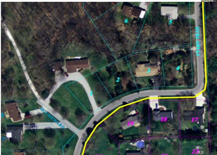
Aerial photograph with proposed Force Main alignment
